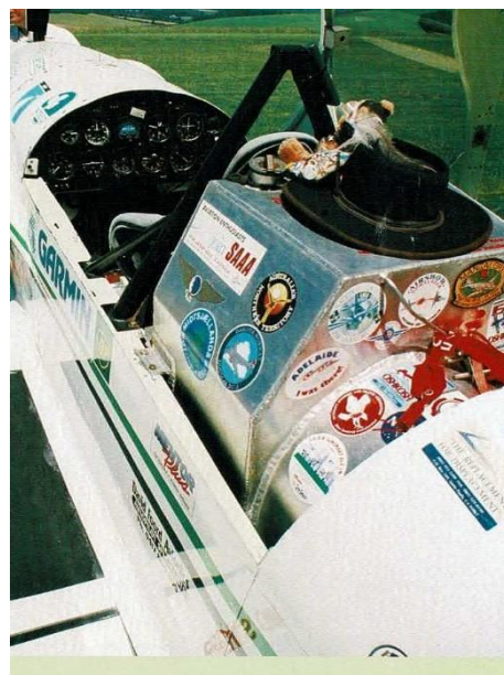
Figure 6 - VH-NOJ at Cranfield showing the fuel tank Jon installed in place of the rear seat [SAAM collection]
